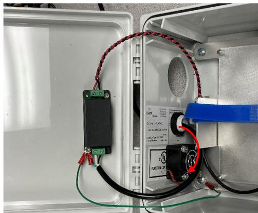
5. Secure the white and black wires of your AC input cable onto the green 2-pin input terminal of the AC/DC converter as shown in the red rectangle below (note that the black wire is on the right of the white wire for the orientation of the photo here). Be sure to tighten firmly.
