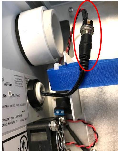
10. Undo the blue Velcro strap. Connect the PAM power connector to the PAM (left photo below). Carefully lower the PAM into the enclosure, being sure that the power connector is securely attached and also ensuring that the PAM is properly positioned over the four mounting posts in the enclosure (right photo below).
