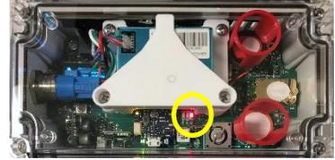
2. Locate the power switch for the PAM. Power on the PAM by pressing the button ONLY ONCE. After a short delay of a few seconds, the button will light up and the PAM will turn on. If the cellular option is present and enabled, verify its green and yellow LEDs are on as described in step 8 of Section B.1.
