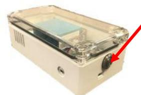
3. Be sure the PAM's inlet and exhaust (on the long sides of the PAM) are not obstructed.
