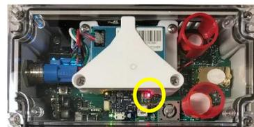
2. Locate the power switch for the PAM. Power on the PAM by pressing the button **ONLY ONCE**. After a short delay of a few seconds, the button will light up and the PAM will turn on. If the cellular option is present and enabled, verify its green and yellow LEDs are on as described in step 8 of Section B.1.
