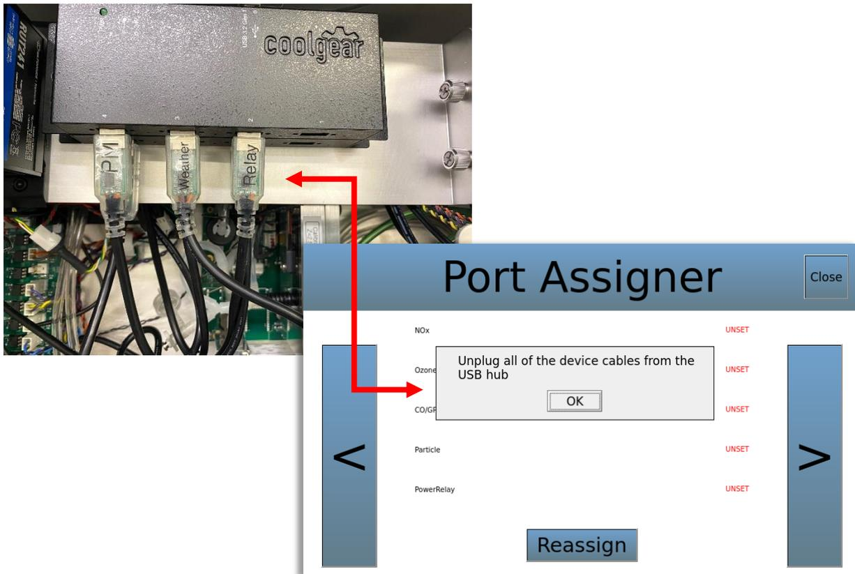
6. Pop ups will start to appear for each device. Plug the USB back into the USB hub making sure you are plugging in the one it requests, and then select yes. For example, NOx is what is shown below.
