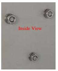
3. Remove the blank weather station power/COM connector by unscrewing the nut on the outside of the enclosure. This can be removed with an adjustable wrench. Remove the piece on the inside of the enclosure.
