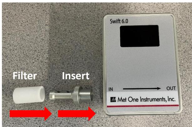
Slide Filter element over the metal insert. Then slide insert fully into the "IN" side of The Swift 6.0 flow meter.
