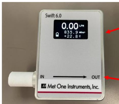
Make sure the flow meter is reading in volumetric flow.
