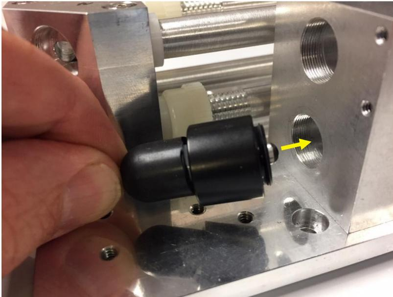
Remove the black light cover for the LED (two screws on the back of the cover). The LED for the NOx instrument is threaded into a hole of the stacked endcap of the instrument's cell. Remove and replace into the same hole on the cell.
