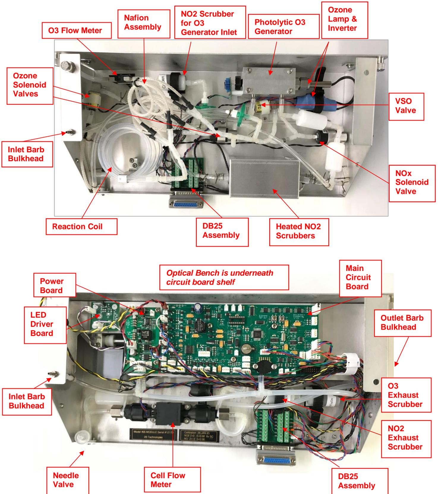
Figure I.5. The NOx Instrument in the AQSync
