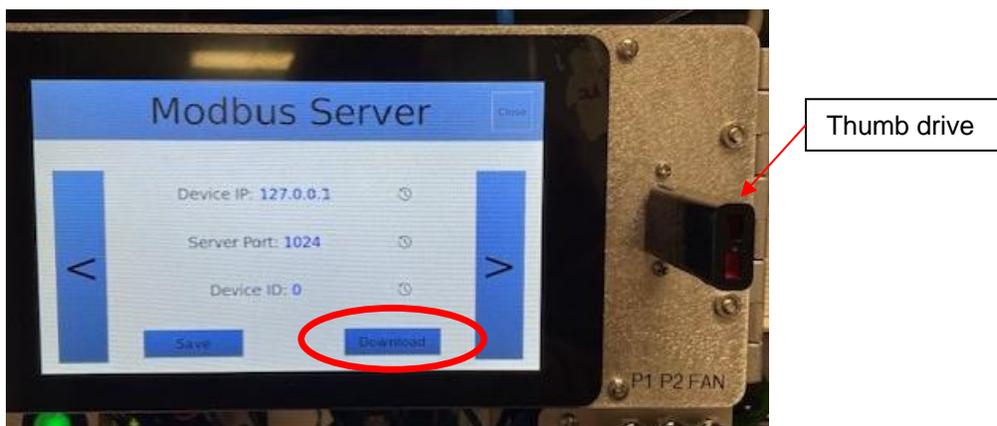
Press "download." The download will take approximately 1-2 min to complete. Press "OK" when download complete. Remove USB thumb drive from AQSync.
