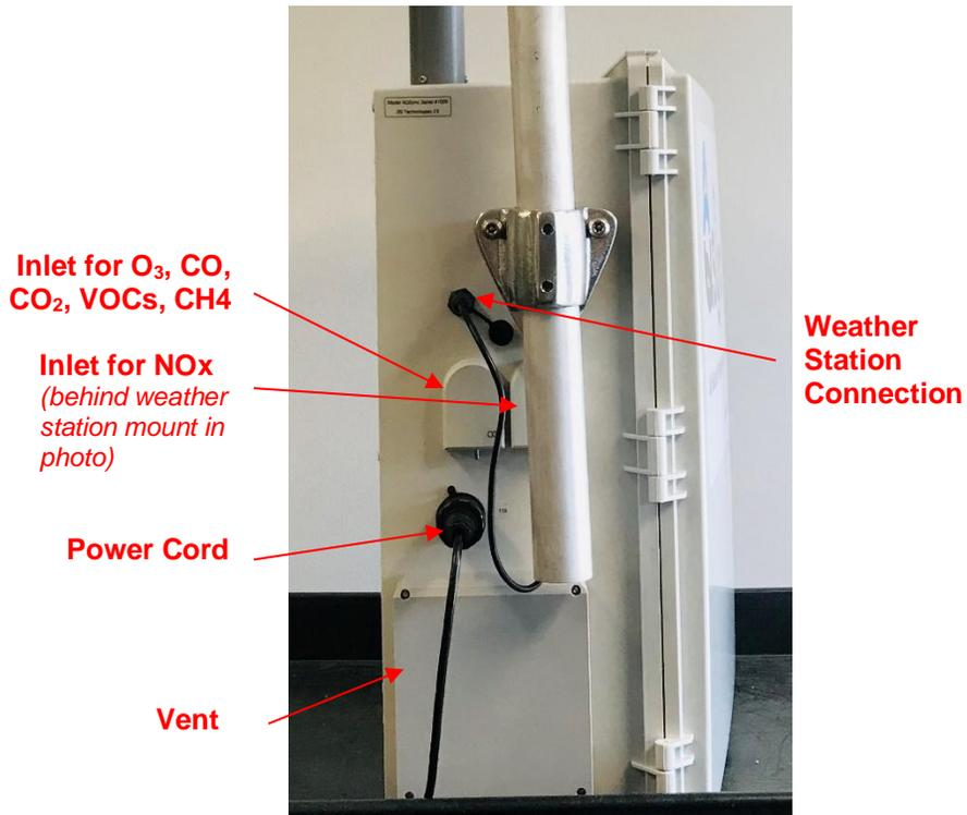
**Figure I.2. Overview of the AQSync Air Quality Monitoring Station**
