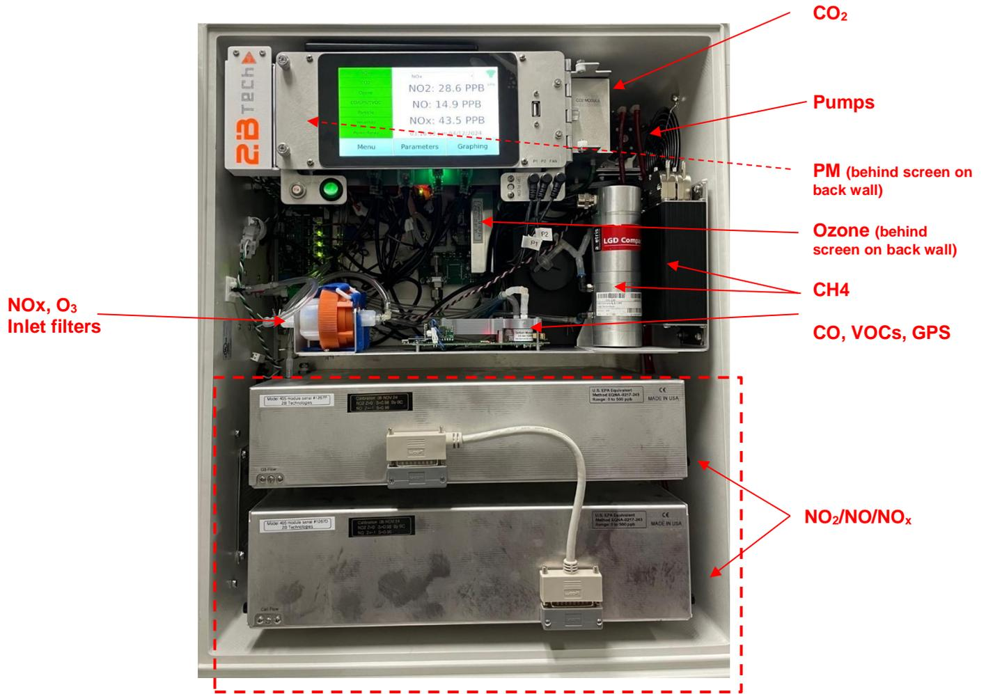
Figure I.3. Overview of the AQSync Air Quality Monitoring Station (inside view)
