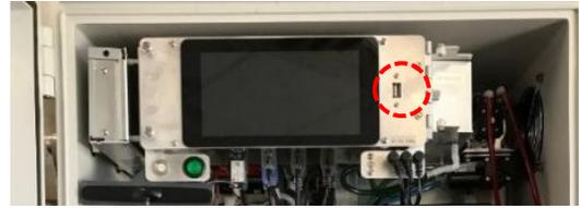
If no USB is connected, the red message appears stating “no USB connected.” When a USB is inserted, hit “refresh.” A green message then will appear saying the USB is connected. ***It is important to “refresh” after adding or removing a USB stick.***
