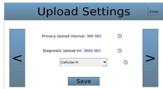
The frequency of the uploads can be specified by tapping on the blue digits in the Primary Upload Interval line in the above right-hand screen. This brings up a keyboard for entering the desired frequency (in seconds). Enter the frequency and select “Save”.
