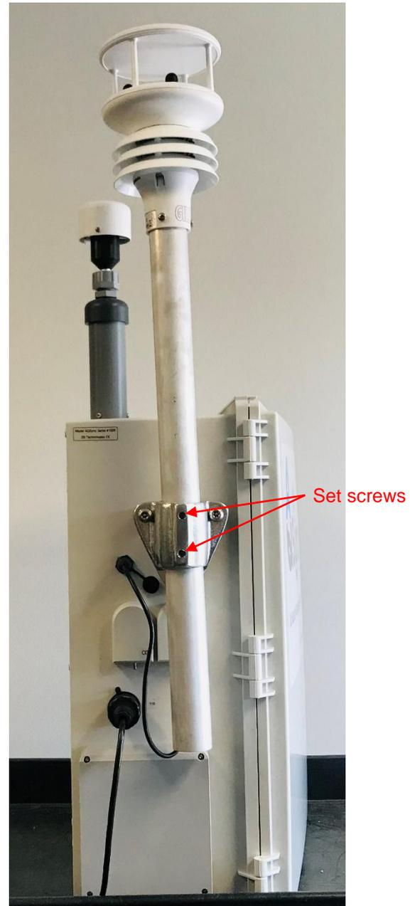
The weather station is a MaxiMet GMX500 Weather Station made by Gill Instruments Ltd. For more information about the installation of the wind sensor, please consult the [manufacturer's manual](#).
