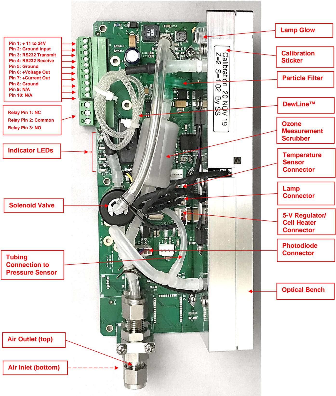
Figure I.4. The 2B Tech Model 108-L Ozone Monitor, the basis of the AQSync's ozone instrument
