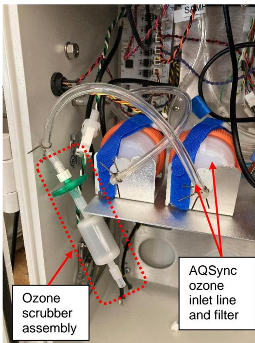
1. Power up the AQSync. For an accurate measurement, the ozone instrument must have been turned on long enough for the internal temperature to stabilize (normally ~20 minutes).
