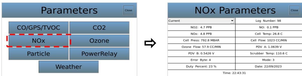
In the above example, values for the NO<sub>2</sub>/NO/NO<sub>x</sub> instrument include the cell temperature and pressure, flow rates, photodiode voltages, scrubber temperature, error byte, and mode. (The [NOx instrument manual](#) and Appendix 1 give more detail about the NOx instrument and the interpretation of this information.)
