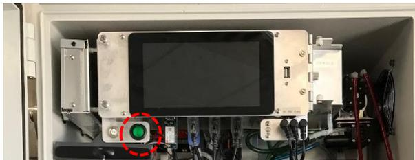
3. The instrument will initialize for a few moments before displaying the main screen shown below. Tap on any parameter on the left to see its current value.
