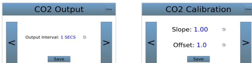
Calibration values for slope and offset (in ppm) can be entered by clicking on the current setting to bring up a keyboard. A calibration for CO<sub>2</sub> is carried out at the factory of the CO<sub>2</sub> instrument manufacturer, and new values would only be needed if a new calibration is carried out by the user or during factory servicing.
