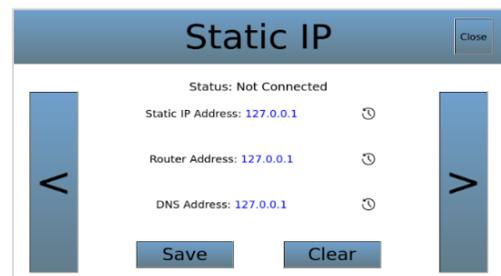
**Warning:** The static IP must be set to a valid IP address and not an IP address which is already assigned to another networked device, or it could cause errors/instrument failure. If you need assistance with this setting, consult your system administrator or contact 2B Technologies' Technical Support.
