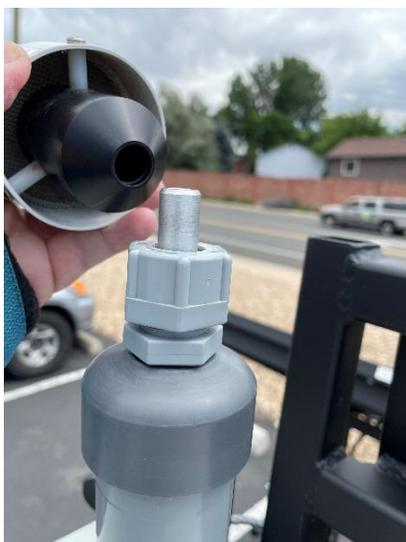
Push the "OUT" side of the Swift flow meter onto the exposed inlet tube.
