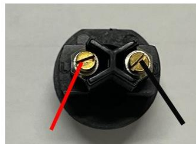
+12V to “L”, -12V “N” on connector
