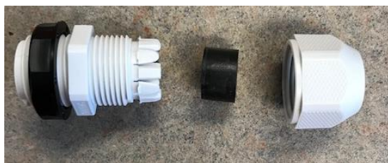
Inside of nut, showing the rubber sleeve with slit
