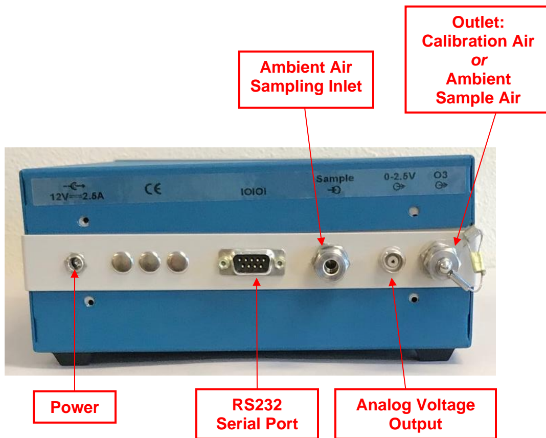
FIGURE 10-4: Back panel of Ozone Cal Source™.
