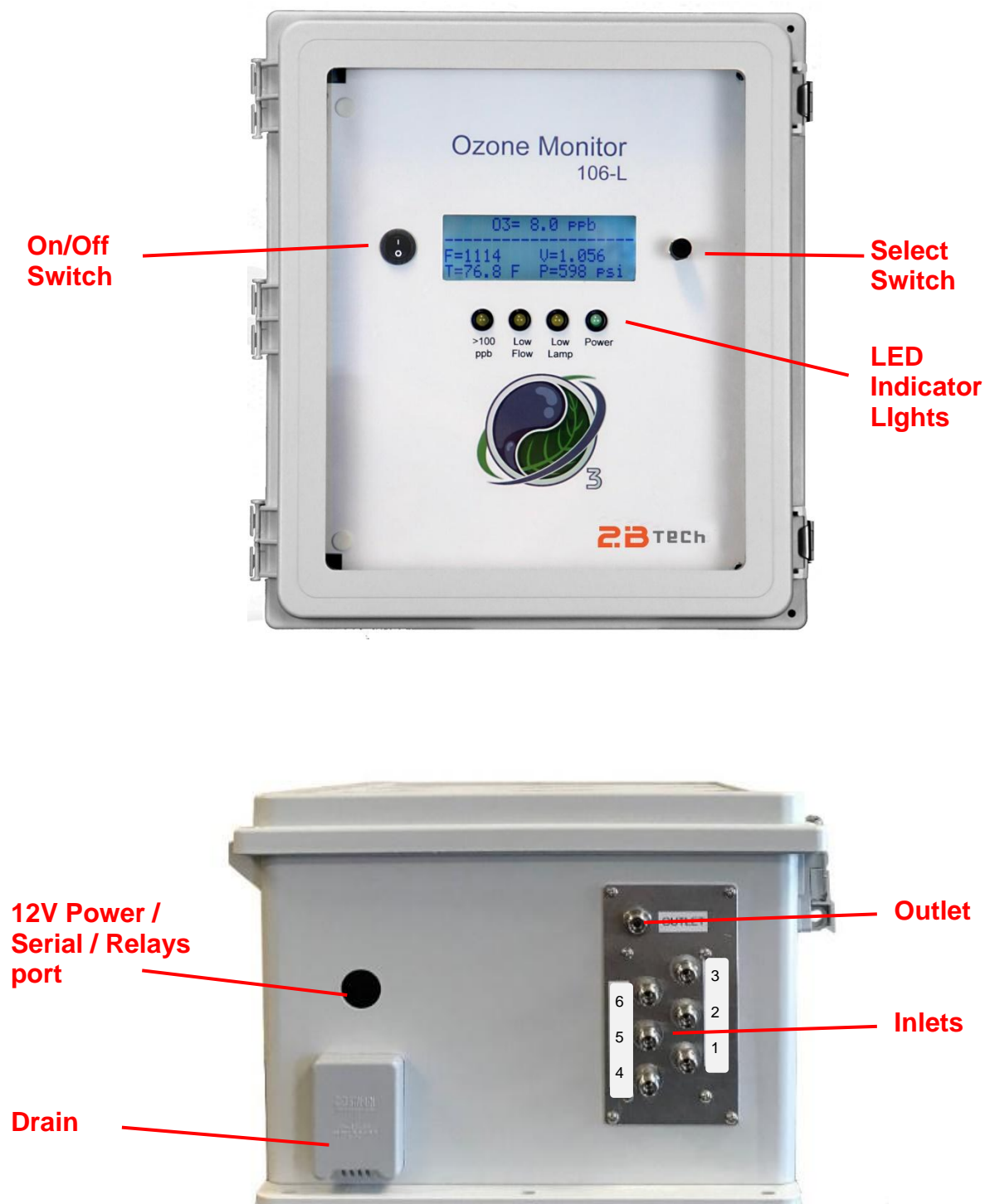
Figure D-6. Front and bottom views of the Model 106-L-MC6 Multi-channel Ozone Monitor.
