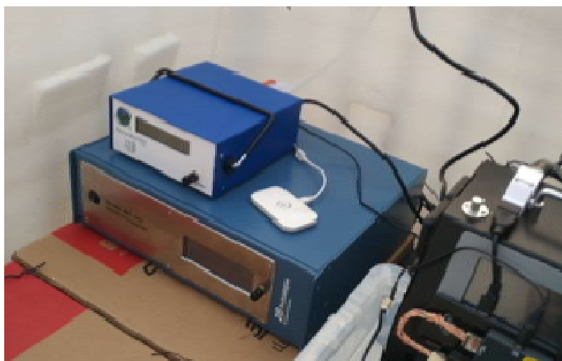
Above: The Model 106-L Ozone Monitor and Model 405 nm NO 2 /NO/NO x Monitor Inside the Moving Cabin
