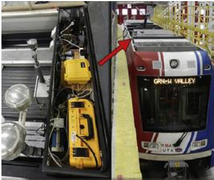
Air Pollution Instruments Installed on TRAX Cars
