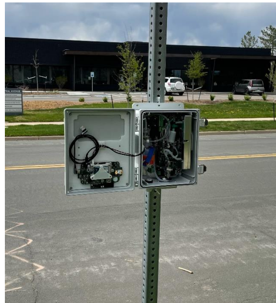
The Model 108-L integrated into a weatherproof enclosure as part of the AQLite Standard Monitoring Package
