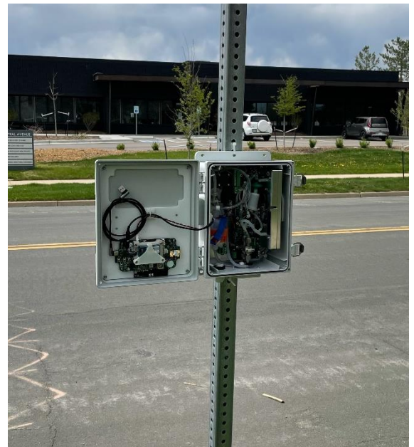
The Model 108-L integrated into a weatherproof enclosure for outdoor monitoring applications
