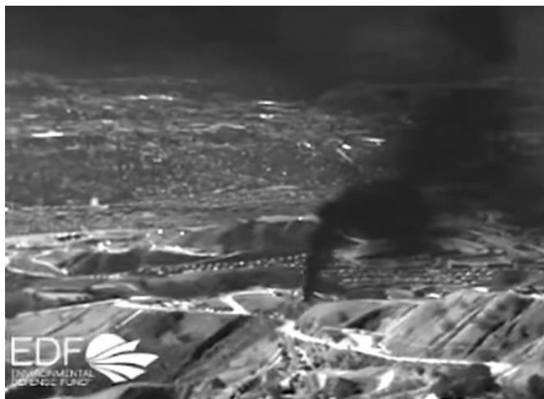
Infrared image of the methane plume from the Aliso Canyon natural gas leak. Image from Environmental Defense Fund. See video of flight around the plume here .
