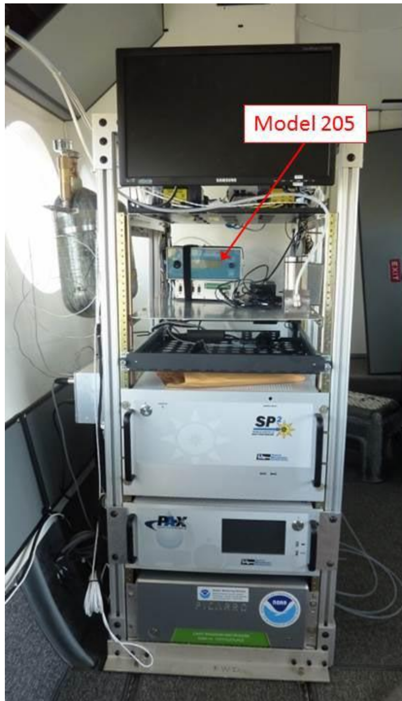
2B Technologies Model 205 Ozone Monitor amidst an assortment of scientific instruments aboard the Cloud Lab
