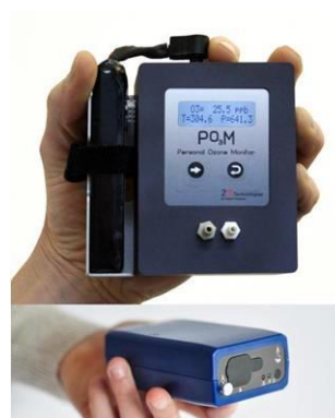
2B Tech Personal Ozone Monitor (top) and AethLabs microAeth personal black carbon monitor (bottom) will be used in the GO3 Treks project.
