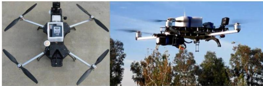
The T&B Systems quadcopter makes use of the 2B Technologies Personal Ozone Monitor (POM) for ozone measurements.
