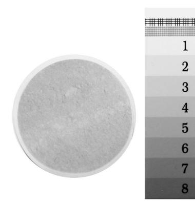
Typical air filter with particulate sample. Students may also estimate the black carbon concentration using a provided greyscale and compare the results to the more accurate nephelometer measurement.
