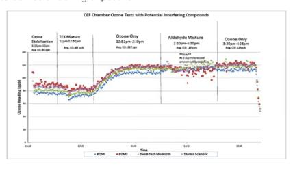
Additional experiments were carried out with exposure to 50 ppb each of vanillin and anisole, food additiives that may be found in indoor air. No differences were found in the responses of the three instruments to these potential UV interferences.
