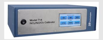
In the Model 714, calibrated concentrations of O3 are produced by photolysis of oxygen, and calibrated concentrations of NO are produced by photolysis of nitrous oxide supplied by a small "Whippit" cartridge. In addition, calibrated concentrations of NO2 are produced by gas-phase titration of NO with O3. Calibrations sequences can be programmed in internal memory via a user-friendly touch screen interface.
